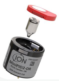
MiniPID 2 HS is designed to detect VOCs at sub ppb concentrations. Detection at these levels can be compromised by contamination from moisture, dust and aerosols. To overcome this, we have developed a world leading, patent pending, filter to protect the ionisation chamber.
