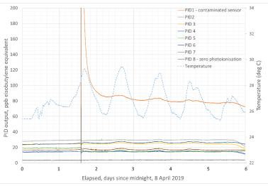
always be undertaken after burn-in using clean air. This will provide the zero point calibration reading. The sensor output with a (masked) lamp delivering zero photionisation is typically 50 and 55 mV (0 to 5 ppb equivalent – see graph above, PID 8).
